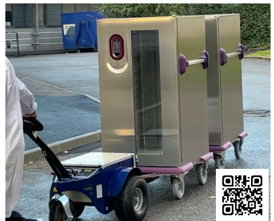
Cabinet towing kit used with a Tractodiff Jobby M4 tractor.
